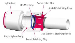
Each socket comprises of an EPDM O-ring, an Acetal retaining ring and a collet (grip ring) containing the stainless-steel grip teeth. When the pipe is inserted into the socket it passes through the collet and the O-ring, to form a seal. The pipe is fully inserted when it reaches the stop within the body of the fitting. The pipe should be fully locked into the collet clip at this point, however, to ensure a tight fit pull the pipe firmly backwards from the fitting.
