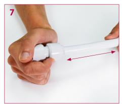
Check the assembly is secure by pulling the pipe away from the fitting.
