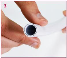
To reduce the risk of leaks, ensure you check the cut pipe is free of imperfections.
